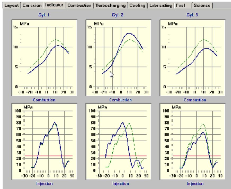
**Fig. 3. Combustion and injection diagrams calculated for different faults (medium speed diesel engine Sulzer3AL25)**
