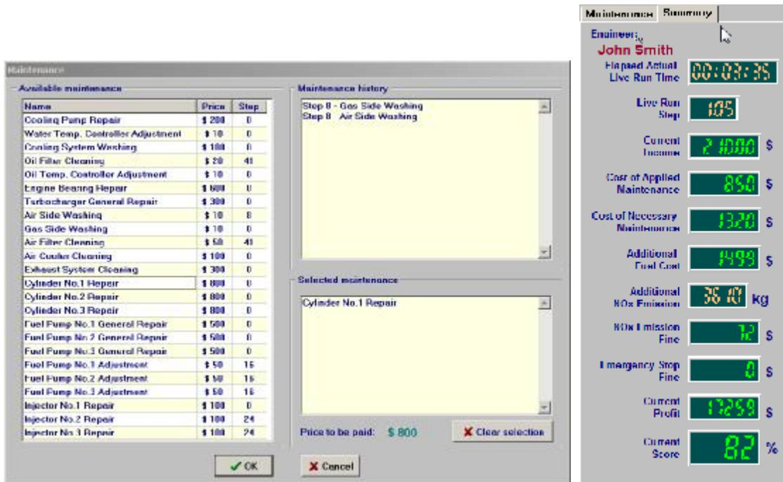
Fig. 5. The choice of available maintenance and repair with their prices Fig. 6. Example of a Live Run current status
