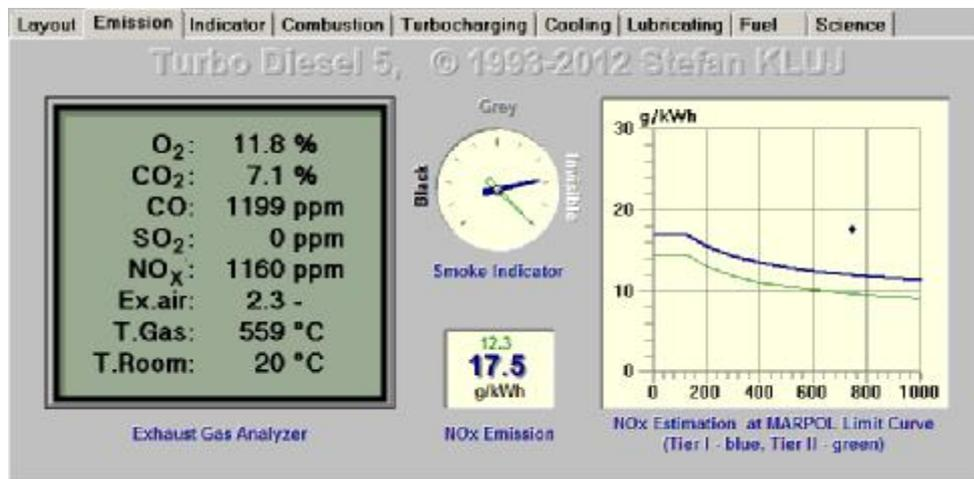
**Fig. 4. Exhaust gas content simulation and its immediate evaluation in reference to MARPOL**
