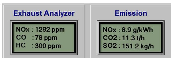
Figure 1. The exhaust analyzer display in VER6 simulator.
