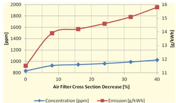
Figure 9. NO<sub>x</sub> emission and concentration as a function of an air filter cross section decrease.
