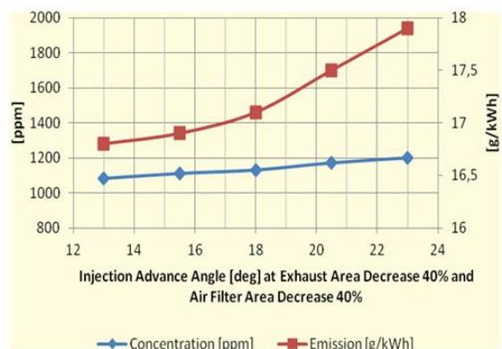
Figure 11. NO<sub>x</sub> emission and concentration as a function of an injection advance angle, dirty exhaust and dirty air filter.
