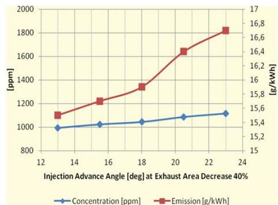
Figure 10. NO<sub>x</sub> emission and concentration as a function an injection advance angle and dirty exhaust.
