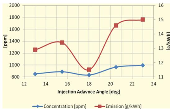
Figure 8. NO<sub>x</sub> emission and concentration as a function of an injection advance angle.
